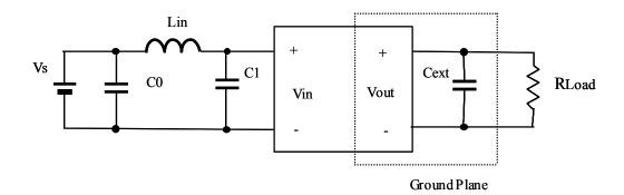
The input reflected ripple is measured with a current probe and oscilloscope. The ripple current is the current through a  $12\mu H$  differential mode inductor, Lin, with esr  $\leq 10$  m $\Omega$ , feeding a capacitor, C1, esr  $\leq 700$  m $\Omega$  @ 100kHz, across the module input voltage pins. The capacitor C1 across the input shall be at least  $100\mu F/100V$ . A  $220\mu F/100V$  capacitor is recommended. A  $220\mu F/100V$  capacitor for C0 is also recommended.
